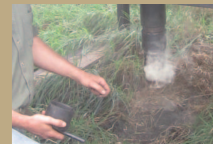
Once the temperature in the kilns reaches 300° the gases begin to escape through pipes underneath the kiln. By capping these pipes volatile gases are redirected into the fire chamber to raise the heat to 600°
